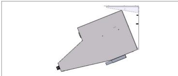
The main unit requires clearance to tilt to a 45° degree angle for maintenance purposes
