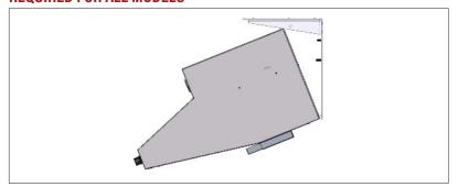
The main unit requires clearance to tilt to a 45° degree angle for maintenance purposes
