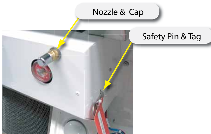
Tank Assembly - Safety Key and Nozzle Assy
